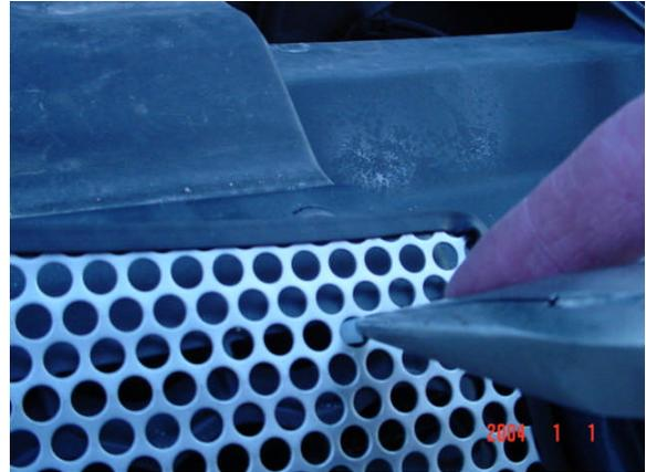
7. Top: Assembles in the same way as the bottom. Apply zipties loosely at first and then snug them up. The grille will protrude under the hood for a clean appearance. This is okay. Notice also that the right side has a notch for your hood latch release. I use 5 zipties on each top piece. The long one is put on in step 8. Two on the top area and 3 along the bottom area.
