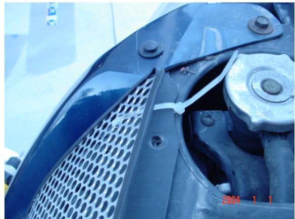
9. Again, draw the zipties snug, cut of the excess, and rotate the lugs out of view.
