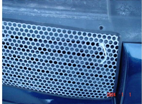
8. The large (long) zipties are used as shown at the right. You can slip the ziptie from the engine bay side through the back of the grille, down one hole and then back through the grille and then slide it under this black plastic piece that you see and then finally back through the ziptie lug. This may require you to remove the screw as shown in the picture to get the ziptie under the black plastic piece.
