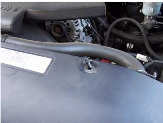
2. Open the hood and you will see a shroud to be removed. Using the small screwdriver pry the push-in fasteners out of the sockets. If you pry the centers up then the sockets will easily removed. Put in a safe place, you will reuse these plugs.
