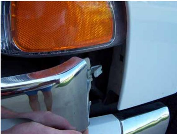
6. To remove the grille, there are 2 clips (1 on each side) below the turn signal. You simply pull while supporting the grille in this area.
