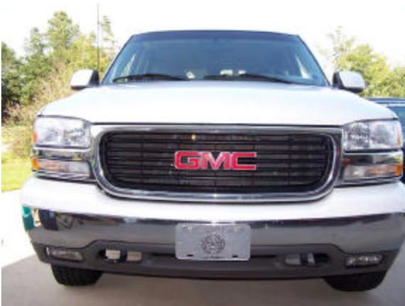
1. This will be our starting point, this is a 2002 GMC Yukon. We provide optional instructions to remount the GMC logo. The small holes in the grille material for the logo must be located and cut by the installer. A simple pair of diagonal cutters or tin snips will suffice. Tools needed: Flat head screwdrivers (1 small, 1 medium), a 10mm socket, and some means of cutting plastic (we used a Dremel tool, but a manual saw will work as well).
