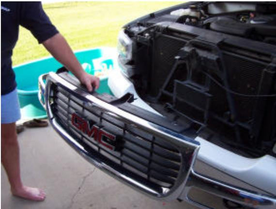
7. The grille can then be removed from the vehicle.
