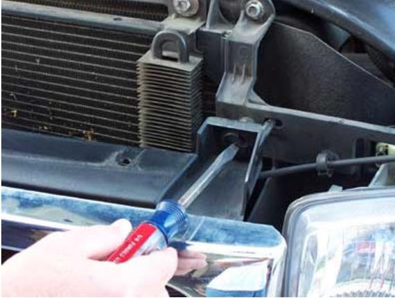
4. Begin removing the grille (plastic chrome) from the vehicle. This is done by turning the quick-lock screws  $\frac{1}{2}$  turn.
