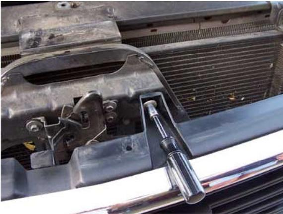
5. Remove the bolt from center, using a 10 mm socket and ratchet or nut driver.
