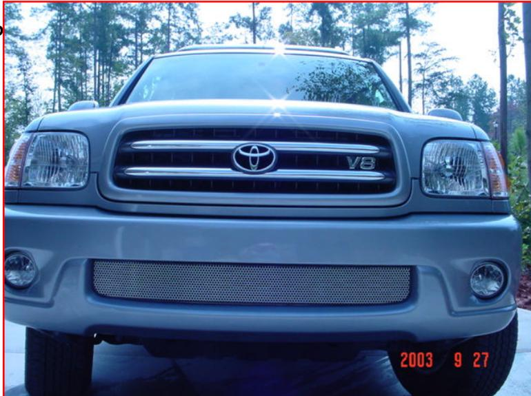
8. Place the grille into position and with one of your hands hold it in position. With the other hand insert a zip-tie from the back of the grill in three locations (one on both sides and one in the middle). After you insert the zip-tie with the lug of the zip-tie on the inside (behind the grille), then feed it back through, tighten it up and clip off the extra zip-tie.
