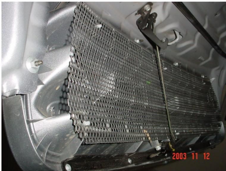
12. Open the hood on your Sequoia and place the grille against the back side of the FACTORY front grille. You will have to slide it behind the hood latch bar.
