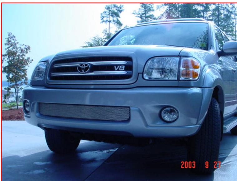
4. Test the fitment of the grille in the lower opening of the Sequoia. Notice that there is a top and bottom as well to the shape of the grille.
