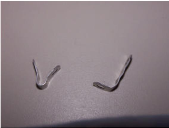
**Step 5:** Bend the brackets to an "L" shape.
