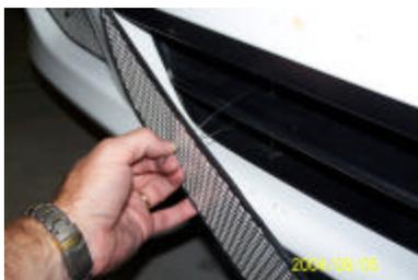
Start at left or right side and push the two ends of the attachment wire through two vertically adjacent holes in the grille that are right in the center. Twist the ends loosely now.
