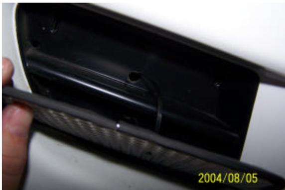
Identify the top and front of the grille. Test fit the grilles on the Odyssey.
