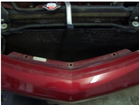
**Step 7:** This is what it will look like with the grille removed. Here you can see the 3 points where the push-in fasteners are located. When reinstalling the grille you will use ty-wraps instead of the fasteners as they will not fit due to the interference with the grille. Below is a pic of our other Odessey grilles.
