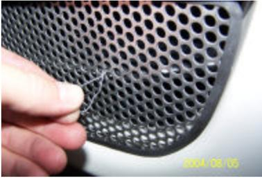
Position the grille to its final position. Now start on one end and tighten the attachment wires and then work your way to all four. Do not overwork the wire or it will break. If so you can get more at Lowes Home Improvement Stores. It is galvanized wire.
