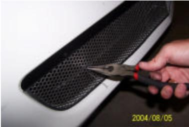
Tighten with needle nose and then cut off the excess. Not too short so it won't come back off but short enough to tuck the sharp ends into the opening where the snips are pointing. Push it easy so you don't break your wire. Wash as you would your car.
