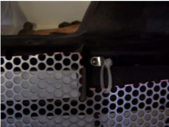
**Step 6:** Use 2 of the screws from the OEM grille and the bracket to attach the grille using ty wraps.
