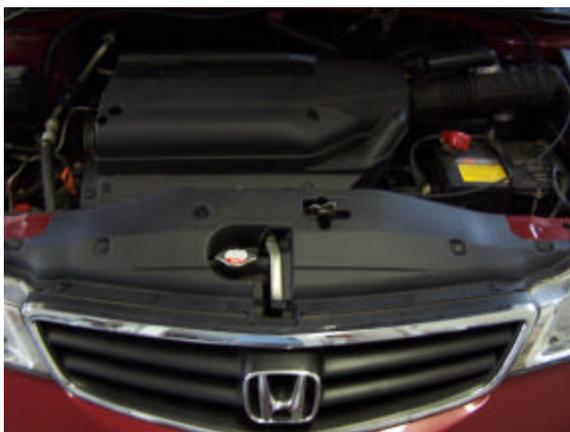
**Step 2:** Open the hood and remove the quick push in fasteners. See the picture to the left. These are removed using the small screwdriver. Be careful or they can be damaged. Good news is you can get them at Lowes Home Improvement Warehouse.
