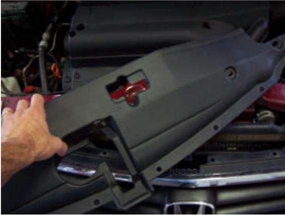
**Step 4:** Remove the shroud, exposing the back of the OEM grille. The grille is now held in by three more of these similar fasteners. They are located on the back at the bottom, where the grille meets the bumper cover.
