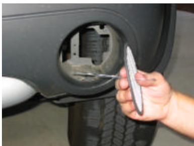
Bend the wire tie and insert it in the center of the grille in two adjacent holes. Then place the grille into the opening and push it in until it hits the two stops (bottom and top). The grille is oval so rotate until you get the best fit.
