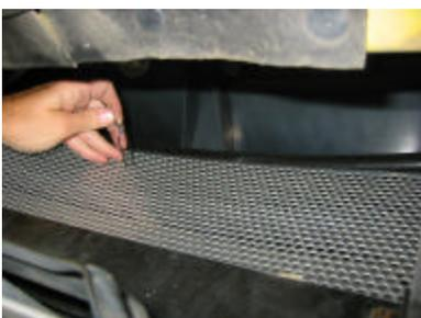
Now you can put the center ziptie through your hole and tighten. This is a photo laying on your back looking up into the grille area from underneath. This is the center ziptie.
