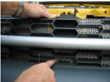
Work it slowly into the inside and move it downward to the Upper grille opening. The notch should rest as shown on the plastic piece in the center.
