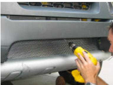
Drill 1 hole into the front bumper (the steel beam) right in the middle. The hole will be angled up slightly. It has to be big enough for the ziptie to pass through.
