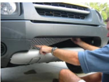
Work it slowly into the inside and move it downward to the lower grille opening. Insert the side with the wider notch first. This may be the left or the right. **Careful with your hands.** Now work the opposite side into place. The notches will get in under the bumper brackets.
