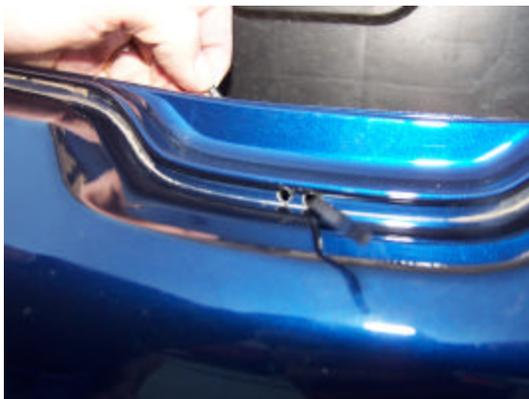
Step 5. Route the tie wrap from the back through one hole and then through the grille and then back through the other hole.
