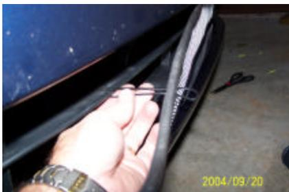
Insert the provided zip ties from the back at the marked holes. Now when you place it back on the car you need to make sure that the ziptie also goes around the horizontal bar from the factory grille so that when you close the zipties they wrap around this bar. You will need to place your arm between the skid guard to reach these zipties and close them with only one-hand.
