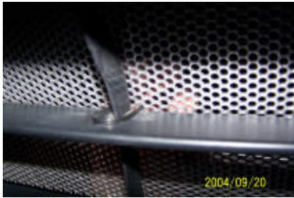
From the back side with you arm slid between the skid guard and plastic bumper, place two zipties through form the back and around a vertical bar (just above the horizontal bar as shown). Then reinsert it through the grille and complete the ziptie from the back side. It takes some practice to do this with one hand. Use the two outer vertical beams to attach to.
