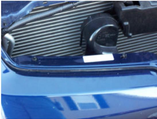
Step 2: Once the shroud is removed, the Upper OEM grille can be slid forward. Careful as it is being held by some fasteners from the bottom. Two of them are seen in the photo to the left. You will want to remove these after the OEM grille is out and put in a safe place.
