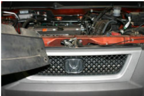
1b. This is a picture showing the plastic shroud being removed. The light grey trim and the black mesh will come off next as an assembly. There are some Phillips head screws from the back. You will need the stubby or a right angle driver to remove the two that are at the top. Note: they are located at the edges. It can then be removed by pulling it forward to release it from the ribs along the lower edge.
