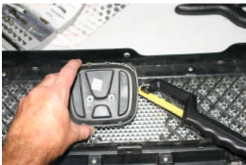
2. Separate the light gray trim from the black honeycomb like mesh. This is done by removing the numerous screws on the back side of the grille (can only be done off of the vehicle). Then using a Hack saw blade (you can use just the blade or a Dremel but be careful) cut the mounting for the Honda emblem (H) out. It will look like this when done. Remove the "H" from the mount if you want to epoxy it back on later.
