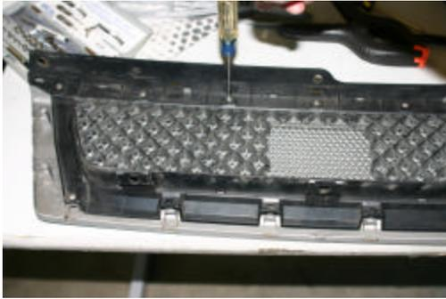
3. Place the GrilleGuy grille on the mesh grille. If any of the gibs (risers that mate the trim to the mesh piece) are obstructed you will need to trim the grille to clear the obstruction. Place the grey trim on and secure using the screws you removed in step two.
