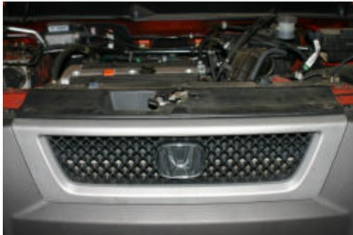
1a. Remove the plastic fasteners that attach the plastic shroud that covers the gap between the grille and the frame. This is done using the flat blade screwdriver by prying the center plug out of the base and then removing the base. If they by chance break you can replace them @ your local home improvement warehouse for mere change.
