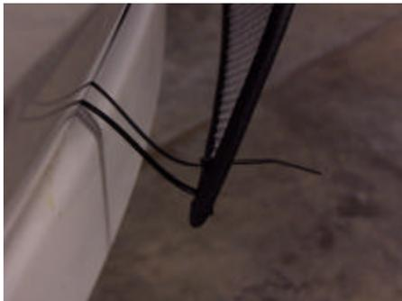
Replace the OEM center grille and then attach the grille using the provided zip ties. You can attach the grille with the method shown (the locking mechanism is directly against the back of the grille, this allows you to pull the zip tie from the front) or just latch the zip ties from the back if you have the upper grille still removed this is simple. We suggest placing the zip ties at the corners and then at the top and bottom at the center.
