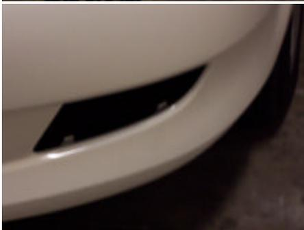
The side vent grilles are removed in the same fashion as the center grille. To access the gibs either reach thru the front opening, the top, or from beneath. Once free from the gibs simply rotate the grille so that it will fit thru the opening.
