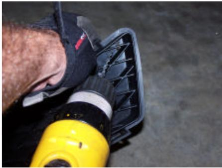
To attach the grille to the side vent, 6 holes need to be drilled. Use 1/4" bit to drill the 6 holes in 3 sets of 2 placed in the corners of the side vent. These will never be able to be seen even if you choose to remove your aftermarket grille.
