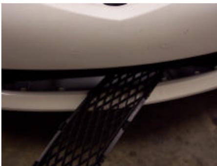
The lower center grille is removed by releasing the gibs and applying inward pressure on the honeycomb. It can then be rotated and pulled out thru the front. **ONLY REMOVE THE CENTER grille** if you are installing the fog grilles. The center grille alone can be installed with the OEM grille in place. For this reason we will cover the fog or side vent grille installation first.
