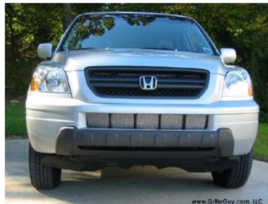
**Step 8:** Replace the OEM Upper grille. Replacing all of the quick fasteners and crimping the clips. To fasten the lower grille you need to remove some of the quick fasteners from the bottom of the car so that you can get your hand behind the grille to fasten the tie wraps. Replace all of the lower fasteners that were removed and your DONE!
