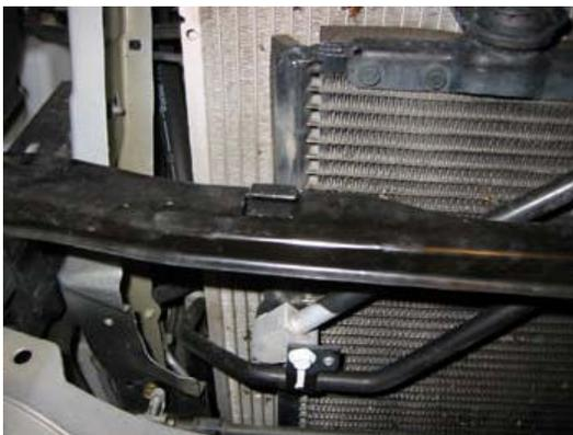
**Step 3:** There are 3 clips that clamp down on some tabs on the back of the OEM grille. You will have to pry these clips open to remove the grille. You will want to crimp these upon reinstall (so don't forget or it will probably rattle).
