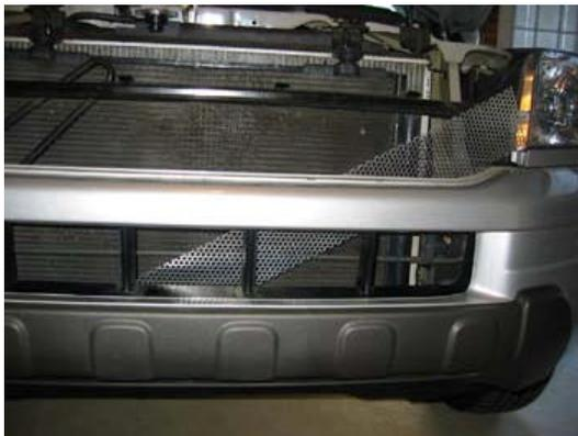
**Step 6:** Place the lower grille in place, but do not attach at this time as you will need to get your hands up through the lower opening to reattach the upper OEM grille. REMEMBER taking it off? You can go ahead and route the toe wraps through the aluminum material at the locations where the vertical bars are located. Some will need to be at the top of the bars and some at the bottom to prevent the grille from moving up or down.
