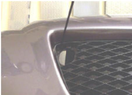
The bottom is attached via a single zip tie located as close to the trim as possible and in the center. Clip all zip tie extensions for a clean install.
