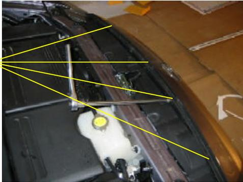
holding the weather trim piece in place. They are removed using a small Phillips screwdriver.
