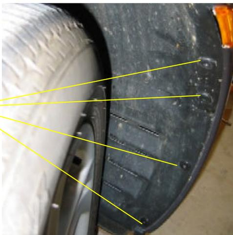
Remove the 4 quick-lock fasteners in the passenger fender wheel (see photo). Using a Phillips head screwdriver, to back the center out (you may need to hold the outer ring to prevent it from turning) then pull the center out and then the outer ring. Repeat this for the driver's side as well.
