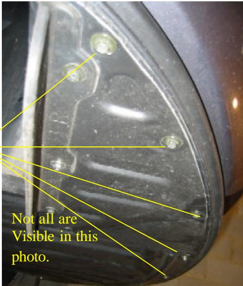
Looking under the front end of the car you will find ten 8mm screws that hold the front bumper to the underpinning (see photo).
