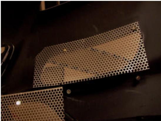
The photo shows the passenger side grille mounted in place. The upper 2 screws go thru the grille material. You will have to align one of the screws and then flex the material so that it follows the contour of the front bumper. Note it will **NOT** be totally flush on the top surface of the fog vent as there is a screw hole that extends up into the way. This will not be
