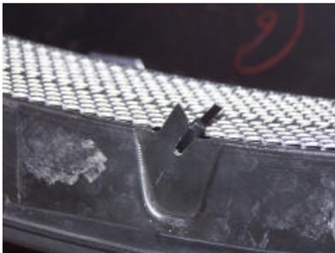
Drill a hole from the bottom in the center of the car. **NOTE:** This hole should come thru behind the "RENEISIS" emblem and will NOT be visible from the front. Check and double check before you drill! Use a zip tie to secure the bottom of the grille to the lower portion of the bumper cover.
