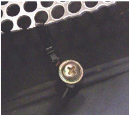
Using 2 zip ties attach the lower portion of this grille. It is accomplished by making a small loop around the screw with 1 zip tie and using the other zip tie to go thru the grille material. Repeat for the drivers side. Note the position of the chamfer will indicate the driver's side from the passenger's side grille.
