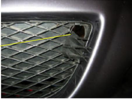
Remove the corner pieces of the main grille by pushing them from the back side and then squeezing the two "tang" of the retaining cord to allow them to be removed. Place these in a safe place; they will no longer be required.
