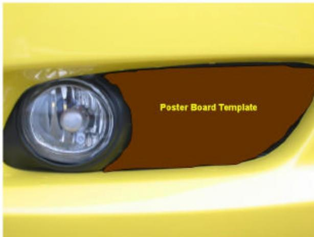
Of course, you want to do a better job with the real thing than I did with the software. Poster board is cheap and easy to cut, so if you have to make several iterations to get a better fit it will be worth it when it comes time to cut the material.
