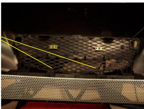
Remove two of the quick-lok fasteners (see photo) center post only and place in a safe place. Route a zip tie through the grille and then through the quick-lok. This will secure the upper portion of the grille. Clip the zip tie extensions for a clean install.
