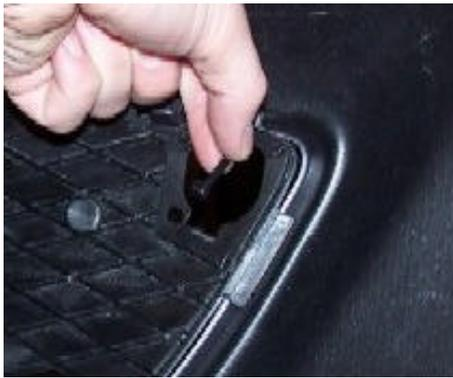
Route a zip tie from the back over top of the OEM grille and then through a hole in the grille and back through an adjacent hole and then through the large opening left from where the piece was removed previously. Do not tighten at this time. You will want to check the fit before snugging up these ties. ***DO NOT over tighten at any point or it could damage the grille!***
