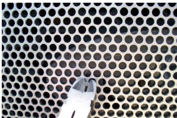
Noting where the stems of the FORD emblem need to go thru, use the diagonal snips to cut away some sections to allow for the stem to go through. Since the Ford Emblem is much larger than the area where the stems are, making the opening larger will not affect the visual appearance. Also there is a pin in the middle that needs to clear as well.
