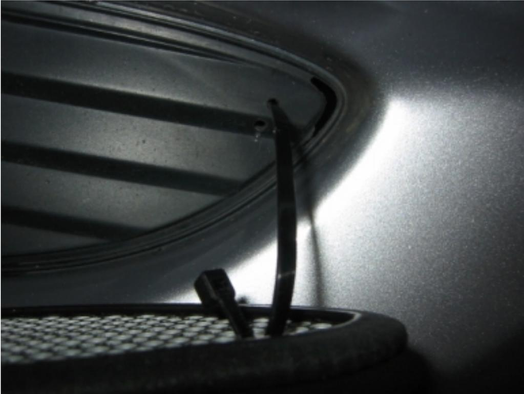
Step 6 - Now, complete the zip tie loop, go ahead and push the zip tie "tail end" thru the back of the grille and out the front. **Loosely fasten the zip tie, do not tighten at this point.** Now do the same for the second cable tie.
