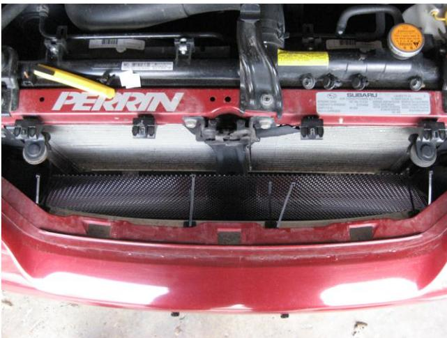
Slide the grille into place and secure the grille to the mounts using the zip ties provided. Tighten only to the point that the grille is secure, no need to over tighten.
