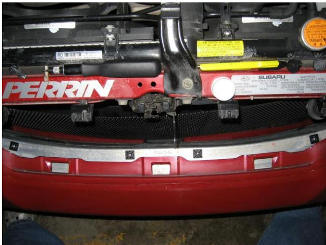
Place 4 mounts on the top of the structural bumper. Again use GOOP to hold these on for best longevity.
