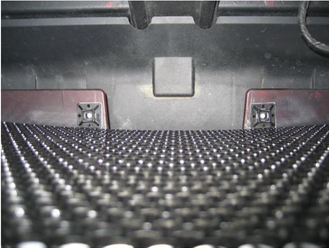
Use 4 more mounts on the bottom of the engine compartment again using GOOP will insure long lasting hold.
