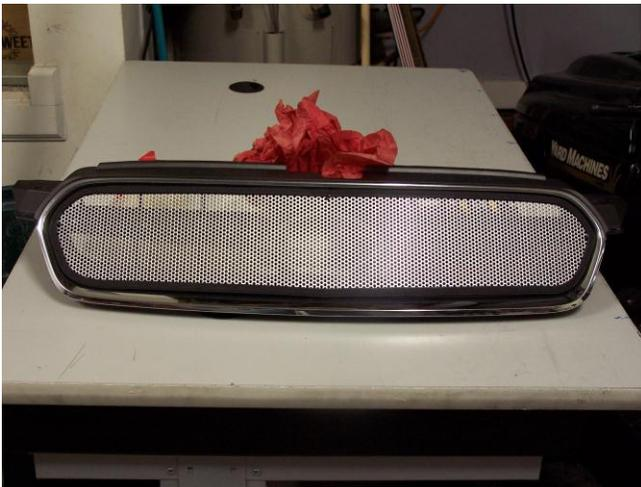
5. The grille is mounted to the OEM grille via the 4 nylon tie wraps. I placed 1 at each end (right at the angle) and then 2 in the center 1 at the bottom and 1 at the top. If you look very closely, you can see 3 of them in this photo. The tie wraps simply loop around the wing and or vertical fins. Do NOT over tighten the tie wraps. Also
