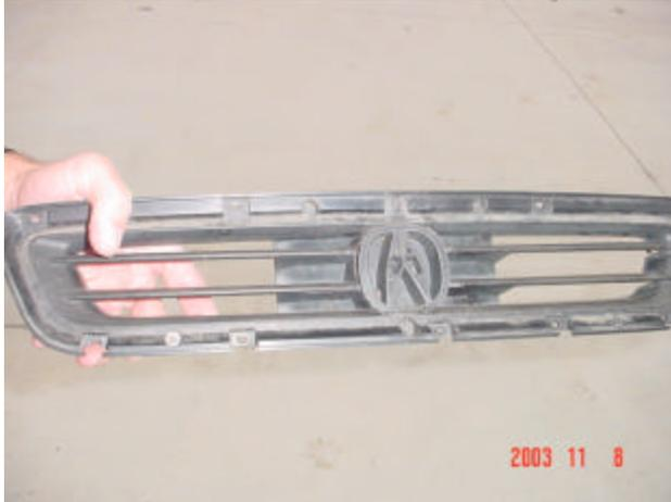
This is what it will look like with the trim removed. You are going to cut the raised section that supports the “A” off so that the grill will lay flat.
