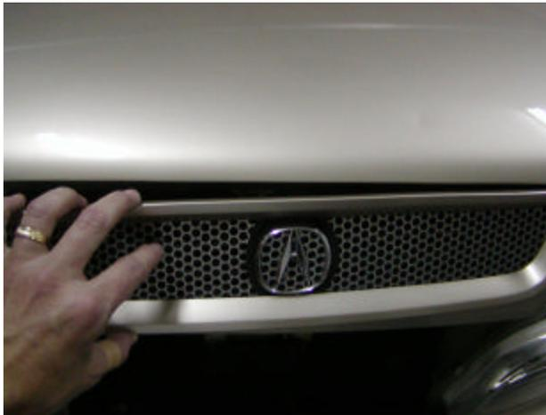
Take the assembly and place back into the hood. You may have to snap the fasteners in using a light pressure at edge of the trim. Replace the 4 nuts on the back and tighten appropriately. Do not over tighten or they could break off! (TOTAL TIME REQUIRED < 40 MINUTES)
