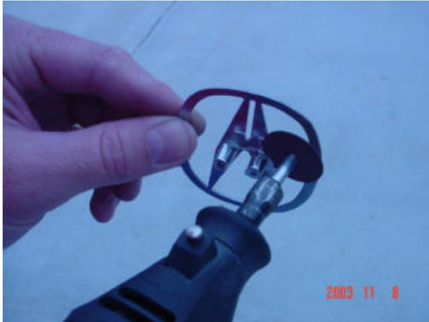
**Figure 8 – Remove the lugs**
