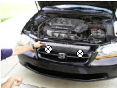
Lets move to the upper grille now so release your hood latch and raise the hood up so we can test the fitment and the bend of the grille. Some tweaking may be necessary for this bend angle. It bends easy so gently bend it to make the angle. The top of the grill should be touching just below the hood latch and the grill should be bent toward the front of the vehicle so it touches the back of the center bar. The top has a notch for hood latch , so you know the top.
