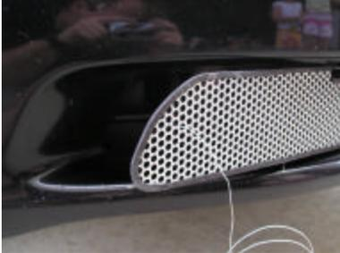
Start with the lower grille. Test the fit and then start at one end and mark either with the wire or with a pencil (or grease pen) the hole that is just above even with the horizontal cross bar of the OEM grille. Do this in at least three locations across the front (Center and ends).
