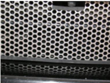
Work from one end and wrap the wire around the horizontal bar and push it back through the hole vertically adjacent (1 above or 1 below). Twist loosely at this point.
