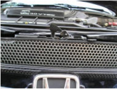
Notice that you need clearance for your hood release latch to get over the grille otherwise you won't be able to open your grille once the hood is shut. This adds a bit of security. Notice we have cut out some to fit under this latch. The rubber trim is to protect your hands from nicks.
