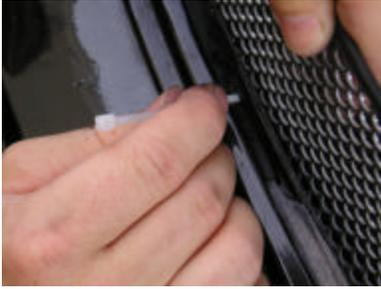
On the center horizontal bar find the slots (marked by the ⊗) in your bumper as indicated with these white zipties. The ziptie will need to be fed from the top of this slot and then feed into the correct hole on the grill. (approx 11 and 13<sup>th</sup> hole down on grill)
