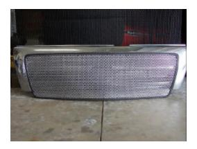
If you want to have the emblem... Remove it from the OEM mount (2 screws from the back) then use some tie wraps or string to attach it to the center (or you can place it it a corner if you want) so that you can mark the grille where you need to cut it.
