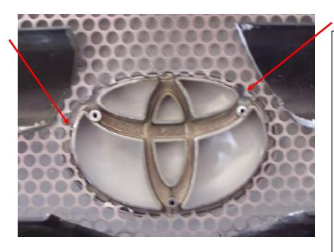
You will note that there is overlap from the outside of the elipse and the front flange. WE will use that overlap to support the emblem. Mark the grille so that the cuts will not be visible outside of the flange, but large enough for the emblem to slide thru. Better to cut too small than too big you can always remove more! Cut using a pair of diagonal cutters, a Dremel, or even a hammer and chisel. Once finished Epoxy it in place with a 5 minute epoxy.
