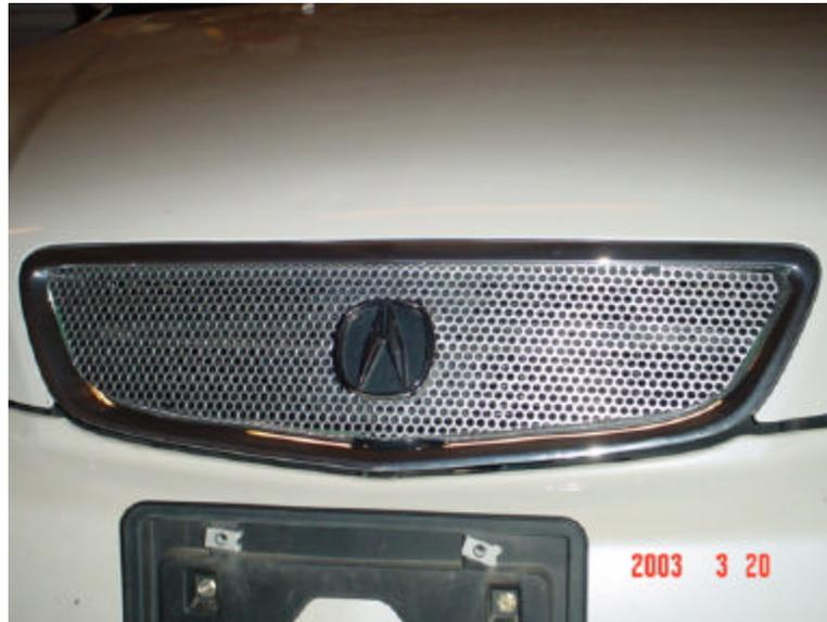
6. If you want to have the 'A' show through then hold the Grille up to your black grille and mark the location of the cutout with a dry erase marker. Make the cutout a little bigger than the mounting boss of the 'A'. We will fill it in with the piece of black rubber enclosed. Please note that your grille shipped with a blue 'F' written in dry erase marker on the front side of the grille.
