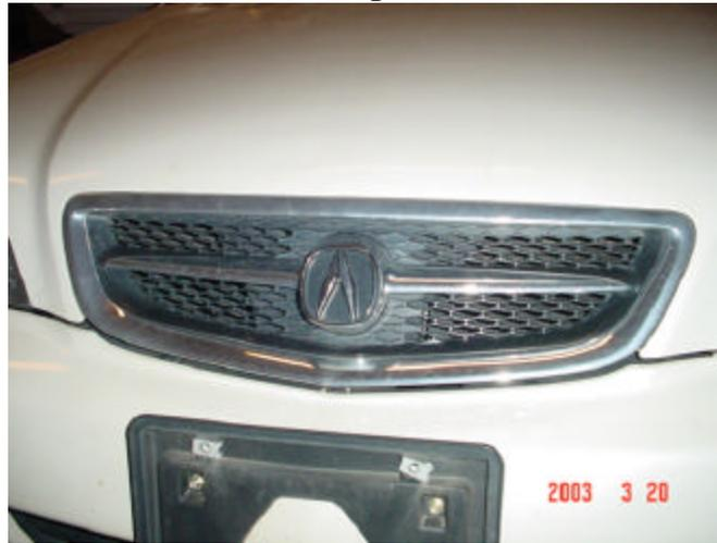
2. Release hood and open the hood. You will notice looking at the back of your grille 5 black cap nuts and two black plastic clips. See photo below. Remove the 5 cap nuts and then while squeezing the plastic tabs pull on the grille from the outside to remove it from the hood
