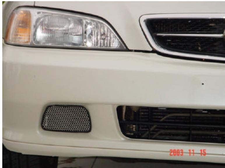
3. Test the fitment of the grille in the fog-light opening of the TL. Note that the bottom edge must go in first to get the angle of the grille.
