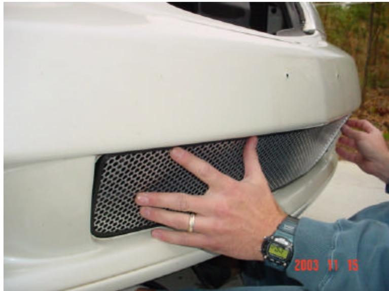
3. Test the fitment of the grille in the lower opening of the TL. Note that the bottom edge must go in first to get the angle of the grille.
