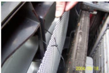
Place grille completely to the left and flush to the front. Find the reinforcement beam that runs VERTICAL behind the grille. Run a ziptie around that beam and then trough the grille. Use holes four holes apart or less and on the same horizontal line of holes.
