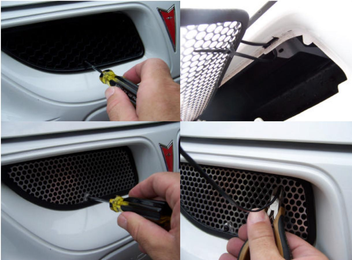
The lower grille is a “put behind grille” and does not require any trim. You will have to get under the front of the bumper to install this grille, you may find it easier to raise the front of the vehicle to do this. However be careful to support the vehicle securely if you do and it is not necessary. Start by holding the grille up behind the plastic lower bumper cover and verify the fit and that you understand how it goes in. The picture below shows how it will look in it’s final position.
