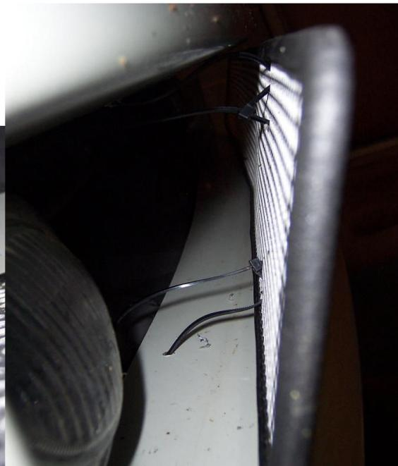
Step 5 – Tighten the cable ties using an alternating pattern. Pull the cable tie tail no more than  $\frac{1}{2}$  inch each time then move to the next point. **This is critical**; if you tighten too much at one time the grille may move out of position in such a way that it can not be repositioned without starting over.
