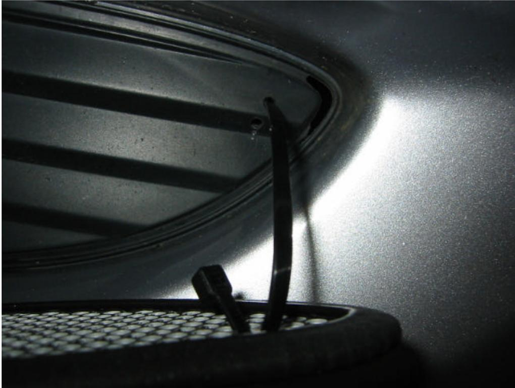
Step 6 - Now, complete the zip tie loop, go ahead and push the zip tie "tail end" thru the back of the grille and out the front. This way you will be able to pull tight from the front side. **Loosely fasten the zip tie, do not tighten at this point.** Now do the same for the second cable tie.
